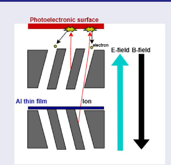
• The time required for ions to reach the photoelectric surface was calculated based on the equations of motion  $m{m a}=q{m E}$
