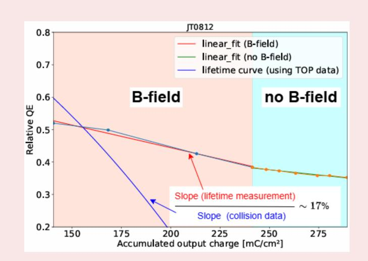
Measurements in a magnetic field suggest that light ions may explain part of the unexpectedly large decrease in quantum efficiency
