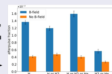
The number of light ions reaching the photocathode was higher under a magnetic field than in the no-field
