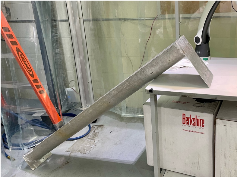
Glue residue after separation
