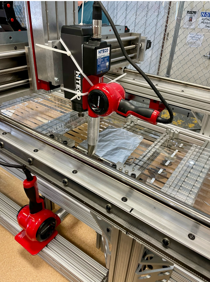
Heat guns softening glue joints between bars
