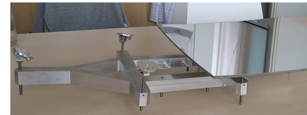
Mirror glueing procedure special glueing table for precise alignment
