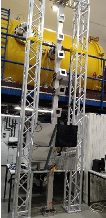
Single pillar + frame prototype with 4 mounted mirror tiles
