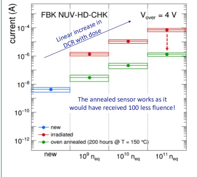
Oven annealing recovers ~97–98% of dark current damage.
