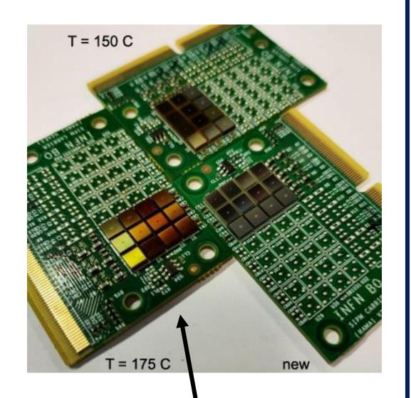
The annealed sensors exhibit a yellowish coloration compared to new ones.
