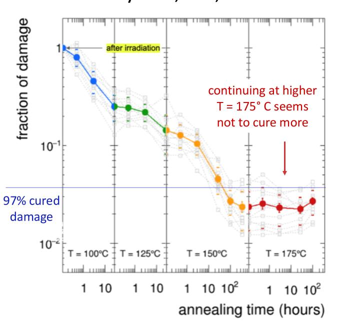
Self-annealing reduces damage
