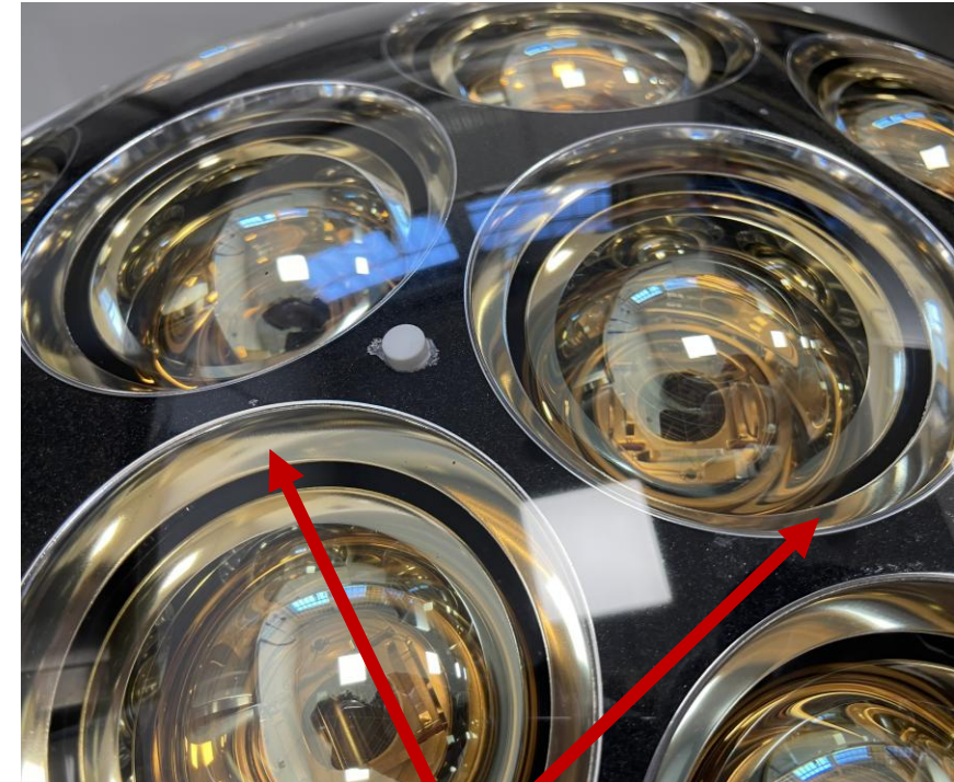
Anodized aluminum reflectors around each PMT
