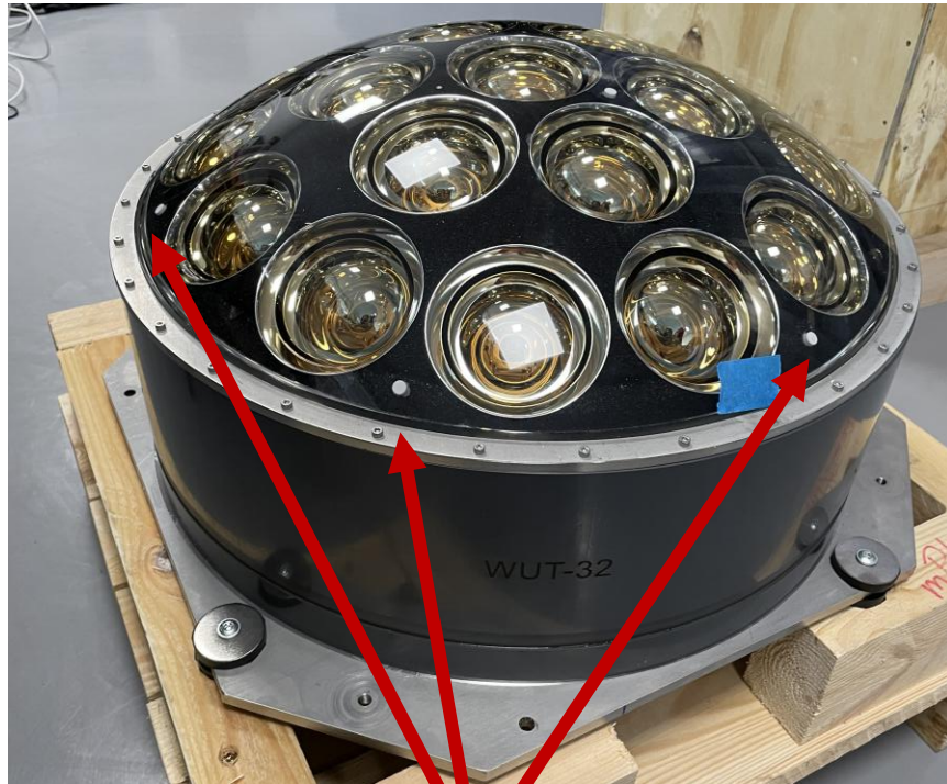
6 slow LEDs fibers output with diffusers
