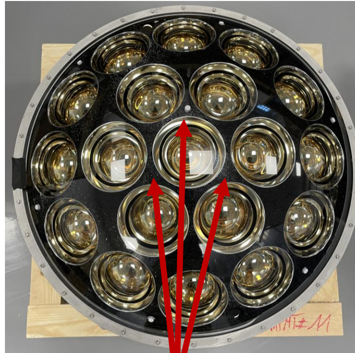
3 fast LEDs fibers output: diffuser, 15 or 30 deg collimators
