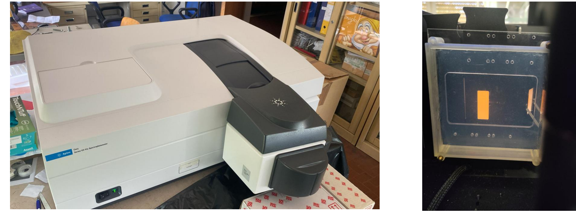
Figure 2. Top view of the Spectrophotometer Agilent – Cary 4000 at INFN Bari laboratories (left); Light spot on the aerogel tile (right).
