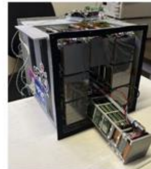
EPIC dRICH prototype SiPM module (INFN Bologna)
