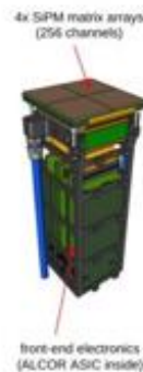
EPIC dRICH prototype SiPM module (INFN Bologna)
