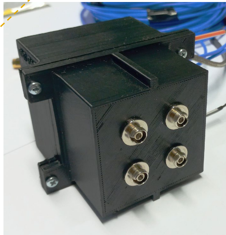
↑ FT0 reference PMT module with a laser intensity monitoring loop and return inputs ↑
