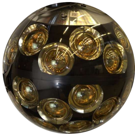
KM3NeT water Cherenkov telescopes: 3D arrays of Digital Optical Modules (DOM)
