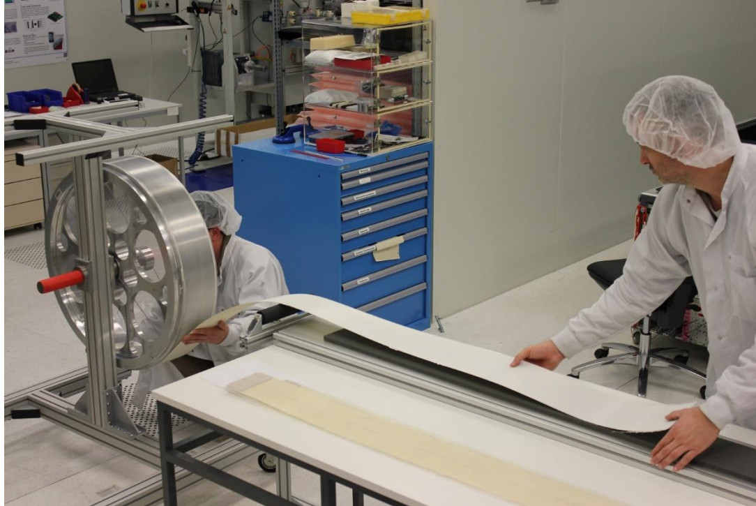
Fibre mat removal from the winding wheel in Aachen
