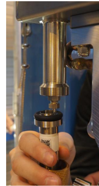
Vacuum bellow with a pin-hole.
