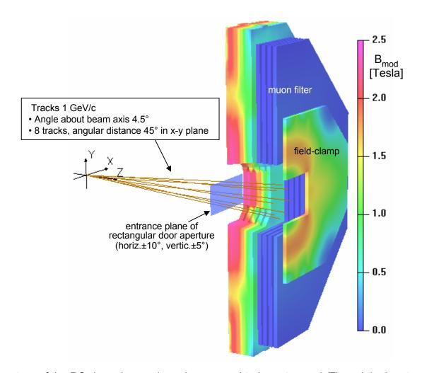
The aperture of the DS-door shown above is assumed to be octagonal. The original rectangular aperture is indicated by a blue plane (the red color in the DS-door, by the way, indicates regions of high iron saturation).
