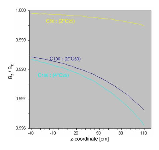
Normalized ratios of axial fields at radius 15 cm for different solenoid currents, labels C100 (full nominal current), C50 (50% nominal current), C25 (25% nominal current)
