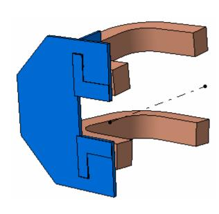
Half of Dipole field-clamp (blue color), fixed to the yoke (which is not shown) Purpose of field-clamp: reduction of magnetic force on Muon Filter, reduction of stray field for Forward Trackers Full dimensions: width ±1.9m, height ±1.2m, thickness 60mm
