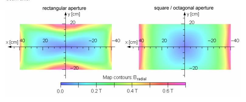
If the aperture would be square or octagonal (see right contour plot) the radial field would increase at the same rate in horizontal and in vertical direction, respectively.
