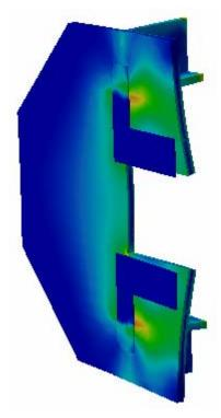
Magnetic force acts mainly at the aperture. There the deflections go up to 0.5mm in z-direction (if no direct mechanical connection to the coils is provided).
