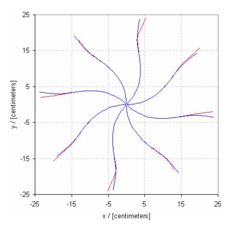
Red tracks: Rectangular aperture of DS-door (±5° vertical, ±10° horizontal) Blue tracks: Octagonal aperture of DS-door (±10° vertical, ±10° horizontal)
