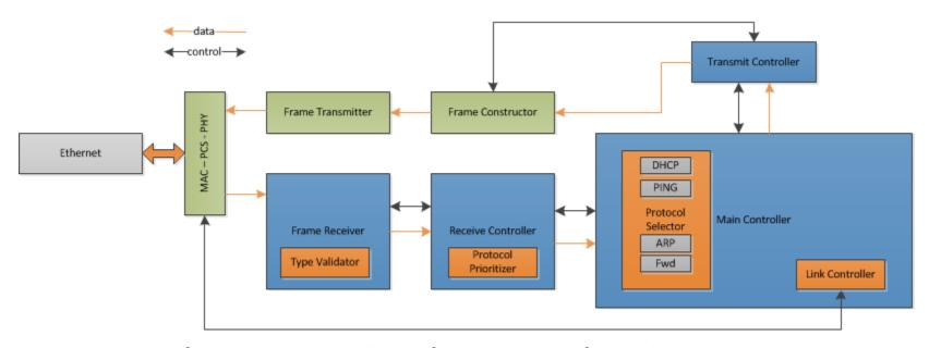
Platform independent framework for Ethernet networks on FPGA devices
