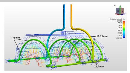
1 bar at the inlet and 0 bar at the outlet applied No significant pressure drop expected
