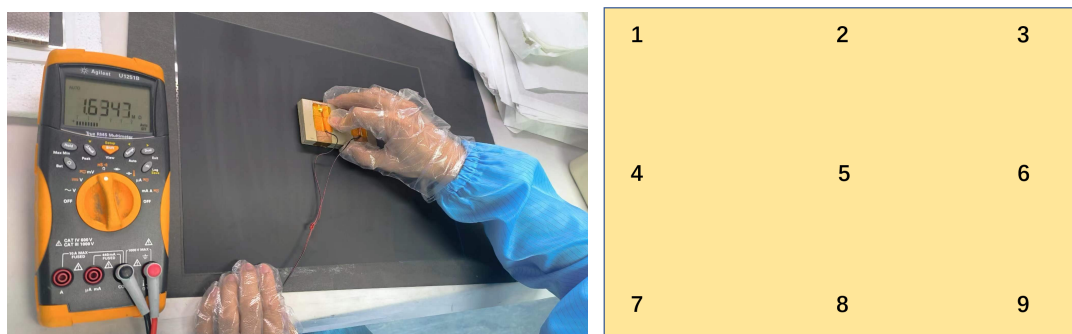
(a) The surface resistance of graphite electrode measurement
