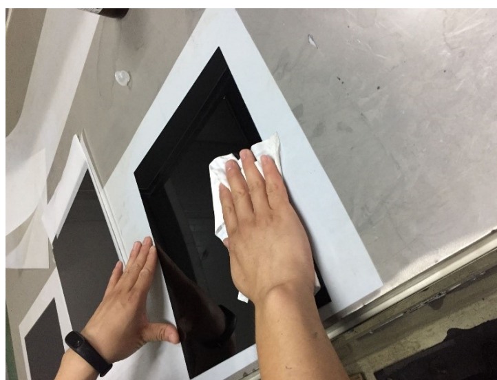
Figure 9: Cleaning the low resistive glass.
