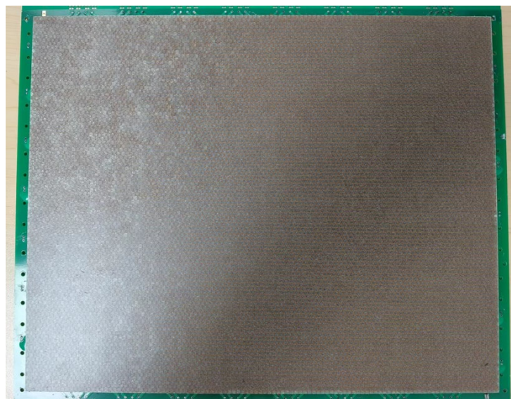
Figure 28: Honeycomb board pasted to PCB
