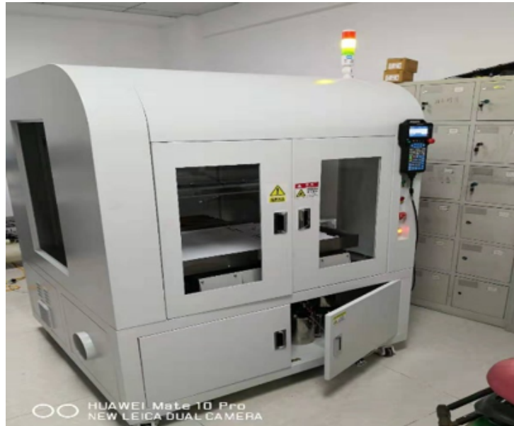
Figure 36: Auto spray machine for graphite electrode
