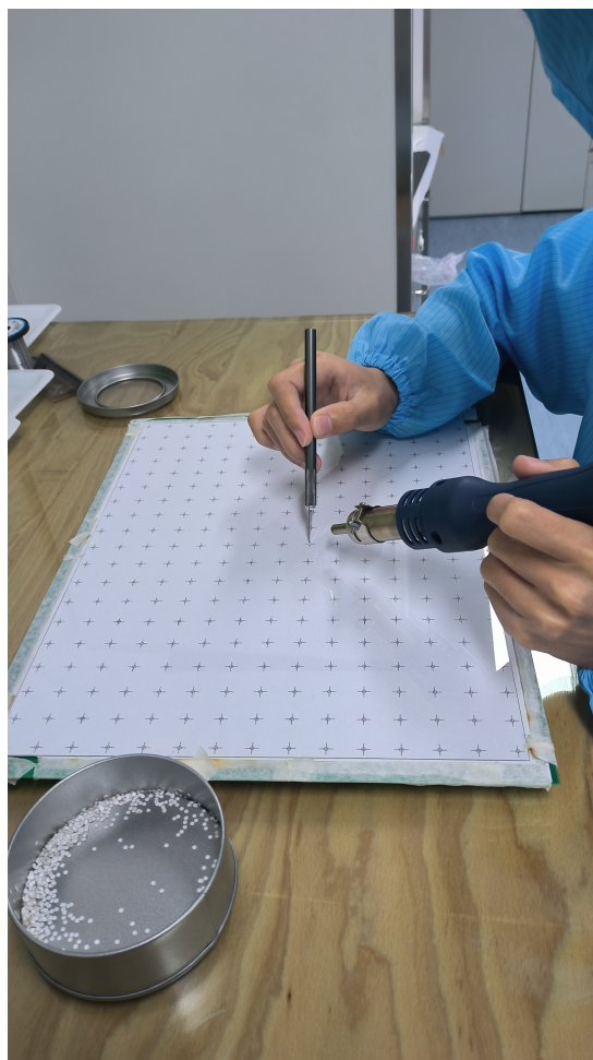
Figure 40: The TBS spacer is being stuck on the glass of MRPC3
