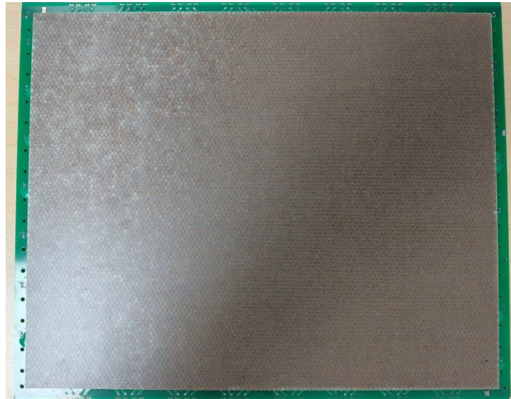
Figure 26: Honeycomb board pasted to PCB
