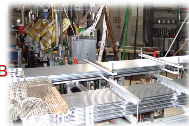
2 straw setups, proton beam coming from the back
