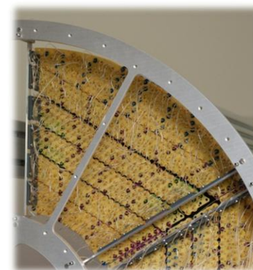
A STT sector consists of 6 straw modules: 2 inner axial + 2 stereo + 2 outer axial
