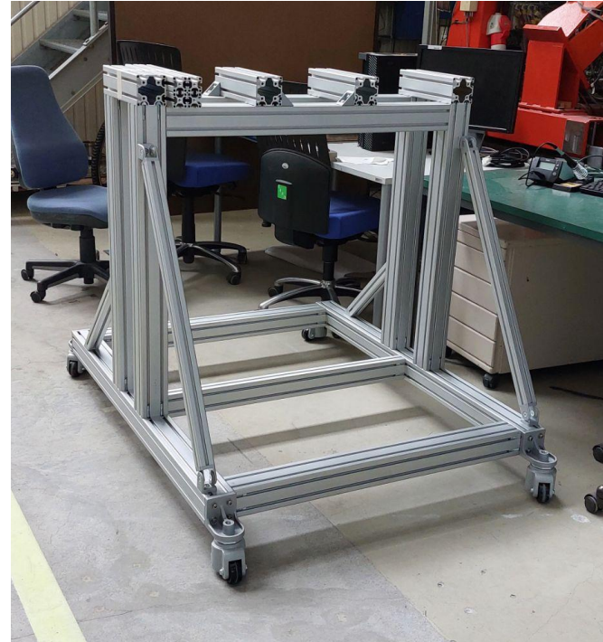
fixed support, ready to install 2 ToFD planes
