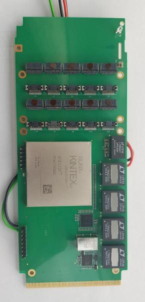
**First** two prototypes using **Megtron 6** (undisclosed manufacturer in China)
