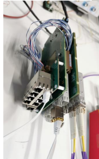
TRB Crate front/back view, TRB3sc in CTS/master/slave setup
