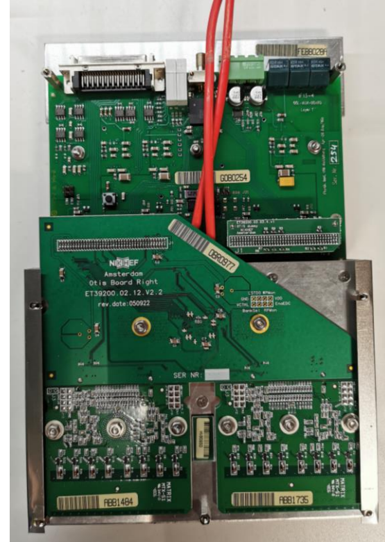
Outer Tracker (half-sized) FEE module
