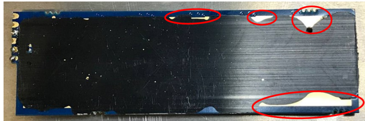
Figure 2.22: Illustration of backplane of FEB, showing an incomplete surface coverage, despite using a well-defined glue application procedure. The encircled areas show the surfaces without glue when the FEB was detached from the shelf.
