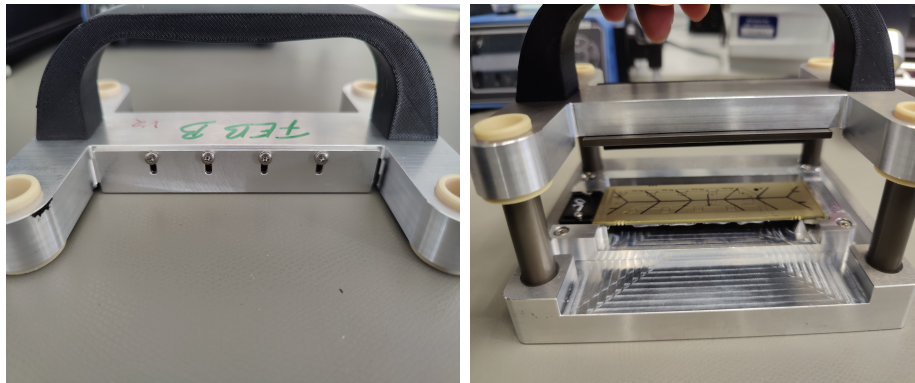
Figure A.1.4: (a) Fixation of cooling shelf with the screws; (b) Sliding down of screwed shelf on the FEB for gluing.
