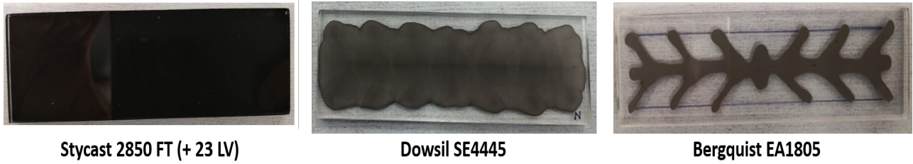
Figure 2.11: The glue samples (left to right) Stycast 2850FT with 23 LV catalyst, Dowsil SE4445, and Bergquist EA1805, showing the surface coverage after the 24 hours of curing time.
