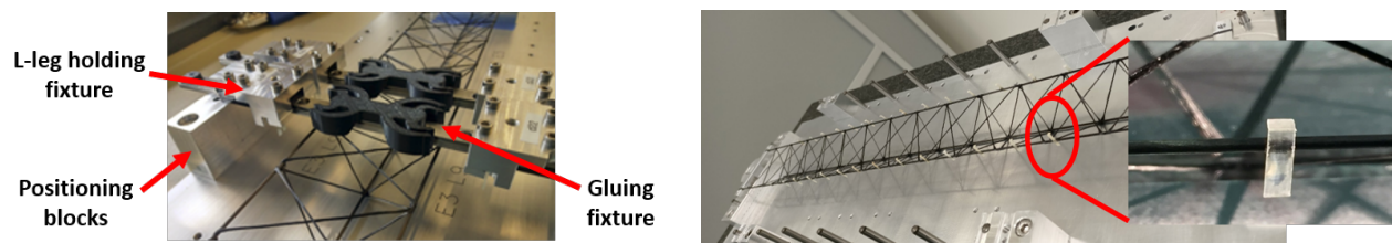
Figure 3.13: (Left) L-leg fixture mounted on the rails, fixed to the positioning blocks, and (Right) L-legs glued onto the ladder after the curing of glue.
