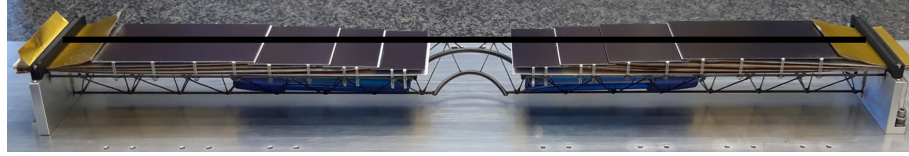
Figure 4.25: Image showing the central ladder with the shift in the perforated tube.
