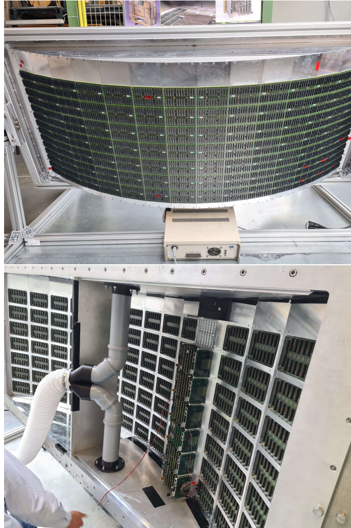
Figure 7.5: The front view of the CBM camera module with all the installed backplanes to hold MAPMTs and DiRICHs (left). The rear view of the camera showing one column of DiRICHs installed to test the cooling system and the section of pipes which will use cool air from a air blower to cool the detector area. The module currently is under tests at Wuppertal.
