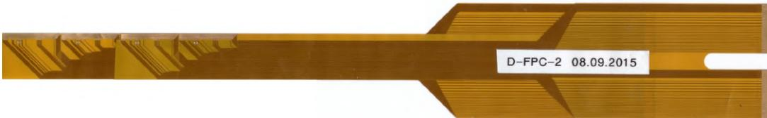
*Figure 2.12: Double-layer FPC for 4 MIMOSA-26 assembled from two single-layer FPCs.*
