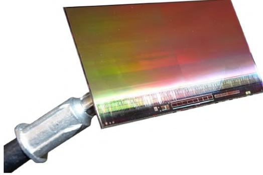
Figure 2.2:  $300 \mu\text{m}$  thick MIMOSIS-1 sensor held with a vacuum pick-up tool. The active pixel matrix is visible in the upper part of the sensor and the passive digital part is visible at the lower part of the sensor [13].
