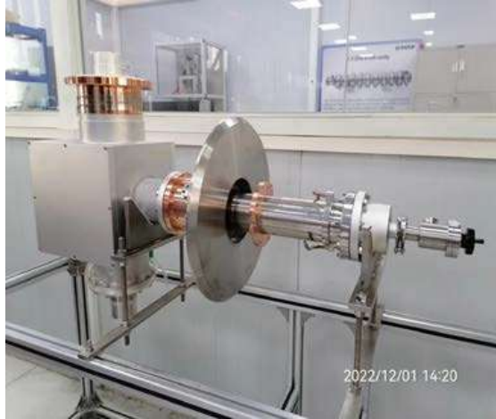
High power coupler and aging test platform
