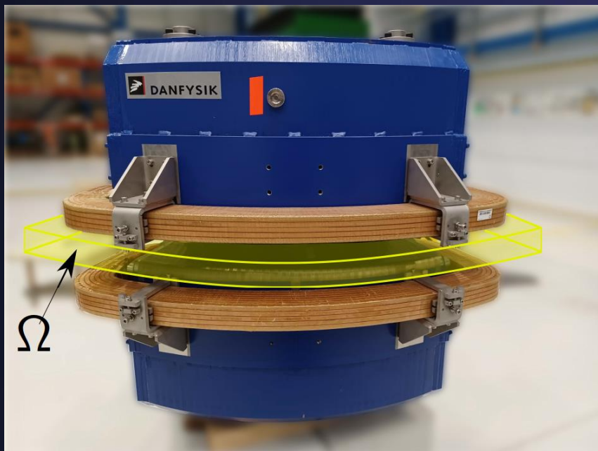
Curved dipole magnet on test bench
