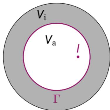
$$\nabla \times \left( \nu_0 \nabla \times \left( \vec{A}_a \right) \right) = 0 \quad \text{in } V_a,$$
