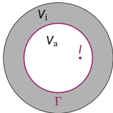
$$\nabla \times \left( \nu_0 \nabla \times (\vec{A}_a - \vec{A}_s - \vec{A}_m) \right) = 0 \quad \text{in } V_a,$$
