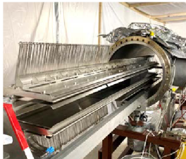
Figure: Damaged wires at SIS18 ES (47% of the length) during beam operation, May 2022, high intensity U, about 4 \cdot 10^{10} ions/cycle. Successfully repaired, 2023 at beam shut-down [1].
