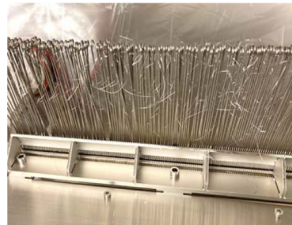
Figure: Damaged wires at SIS18 ES (47% of the length) during beam operation, May 2022, high intensity U, about 4 \cdot 10^{10} ions/cycle. Successfully repaired, 2023 at beam shut-down [1].
