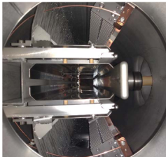
Figure: Damaged wires at SIS18 ES (47% of the length) during beam operation, May 2022, high intensity U, about 4 \cdot 10^{10} ions/cycle. Successfully repaired, 2023 at beam shut-down [1].
