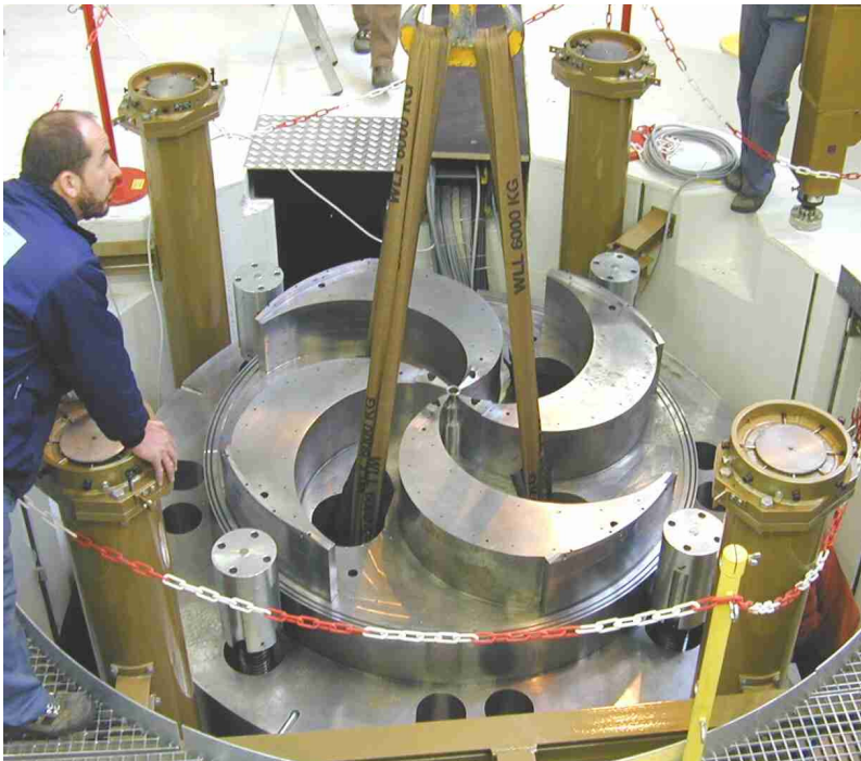
PSI/Varian comet: 250MeV sc. medical cyclotron
