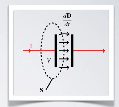
The current used to charge the capacitor equals the rate of change of the charge on a capacitor plate and equals the displacement current between the capacitor plates.
