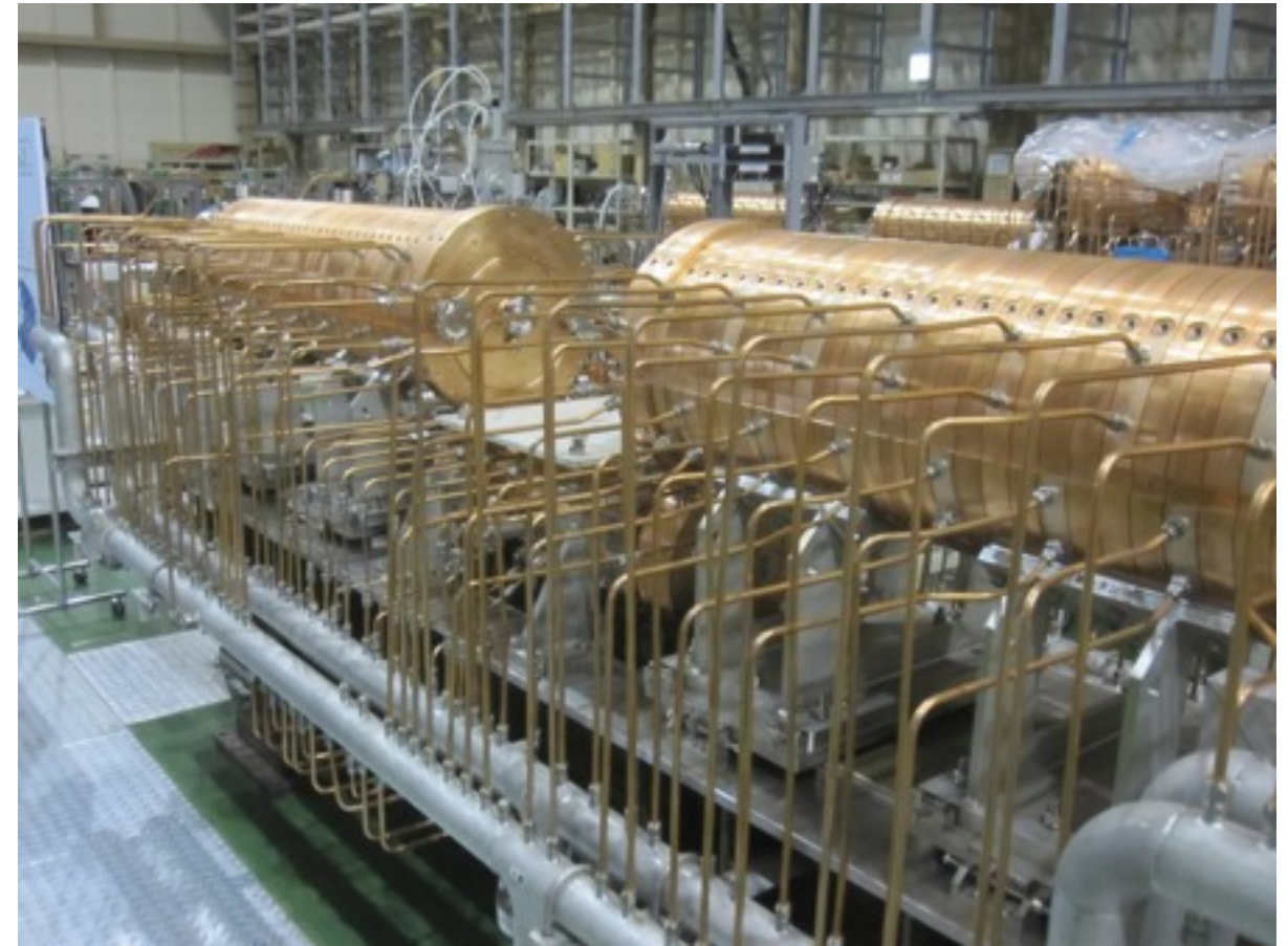
New ACS accelerating structures for 180–400 MeV section; currently being installed.
