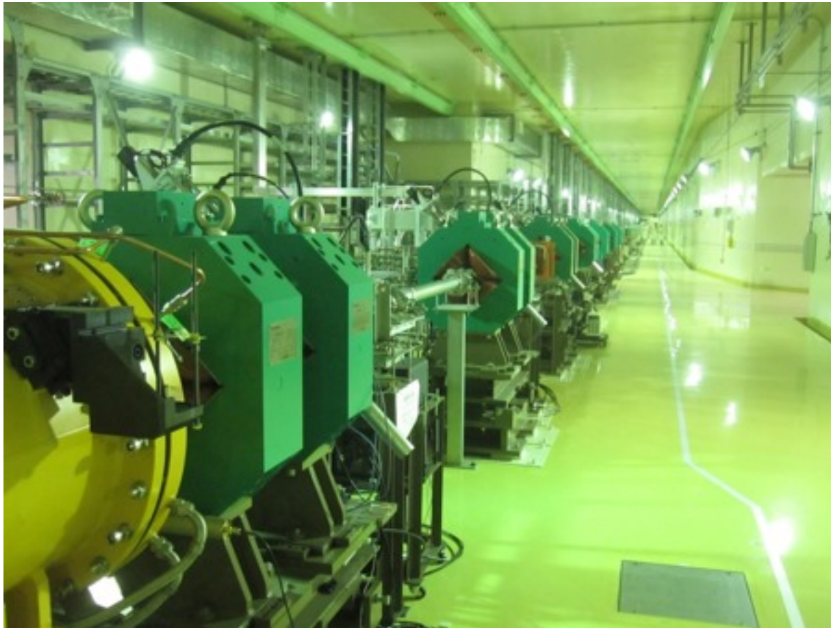
Quadrupole transfer line from 180 MeV linac being removed
