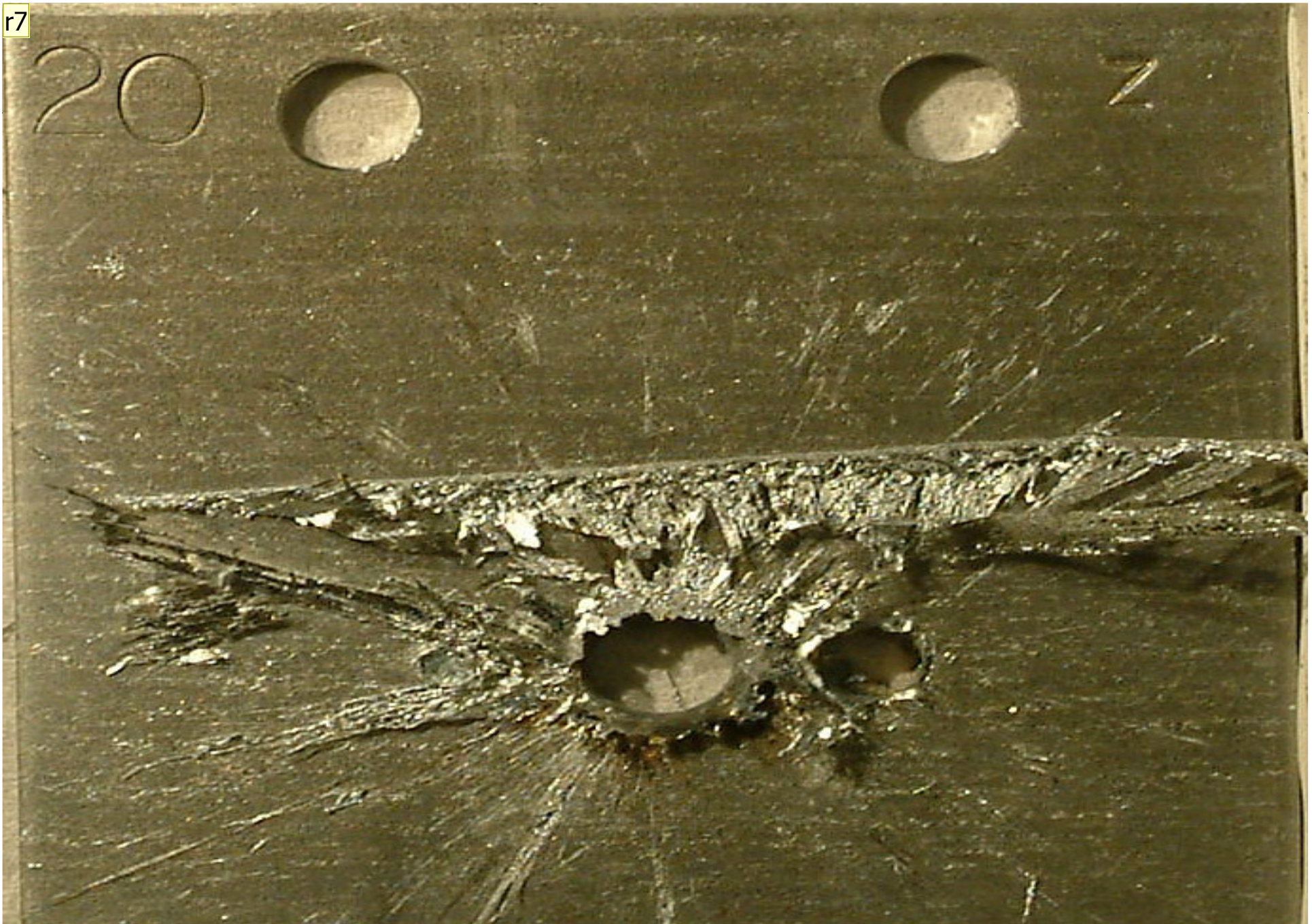
Proton bunches at the end of their life during an SPS test: damage to metal structure
