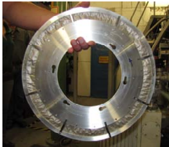
Foil stripper before (bottom) and after (top) high current operation. For the second foil (top, from the right) 11 kJ of beam energy were deposited without any observed influence on the beam parameters.
