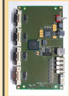
CamLink FPGA board is used for readout of 2-4 cameras.
