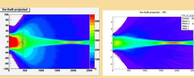
Extrapolated transverse positions of pellet tracks from experimental data taken at UPTS (left) and the result of the simulation (right). The scale on the x-axis is in millimeters. A focus is seen at about 2000 mm which is the position of generation.
