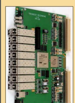
VME FPGA board (developed for the WASA trigger) is used for readout of up to 8 CamLink FPGA boards.
