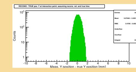
$\rightarrow$  Resolution  $\sigma \approx 0.8$  mm for 4  $\mu s$  effective measurement resolution.
