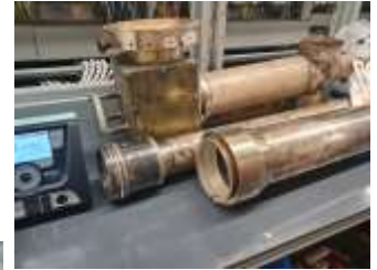
A2A waveguide short. small PTFE ring...
