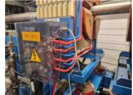
leak copper pipe..., brazed, ... insulated.
