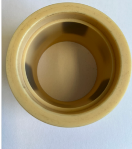
Ceramic isolator after operation with Cr
