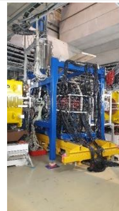
S2 focal plane: Implementation of new, modular support frames for fast and reliable changeover of complex experiment setups
