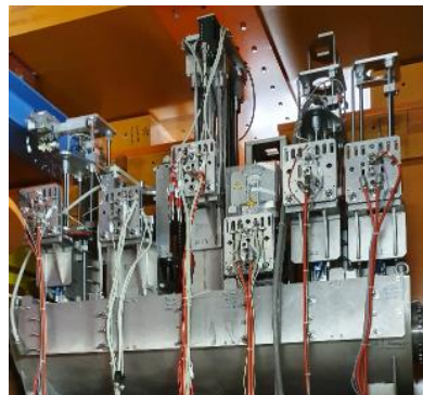
S1 focal plane: Improved separation and identification of secondary beams (new, turnable disc degrader and new TOF system)
