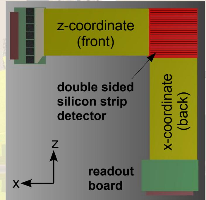
Readout of double sided silicon strip detectors:
