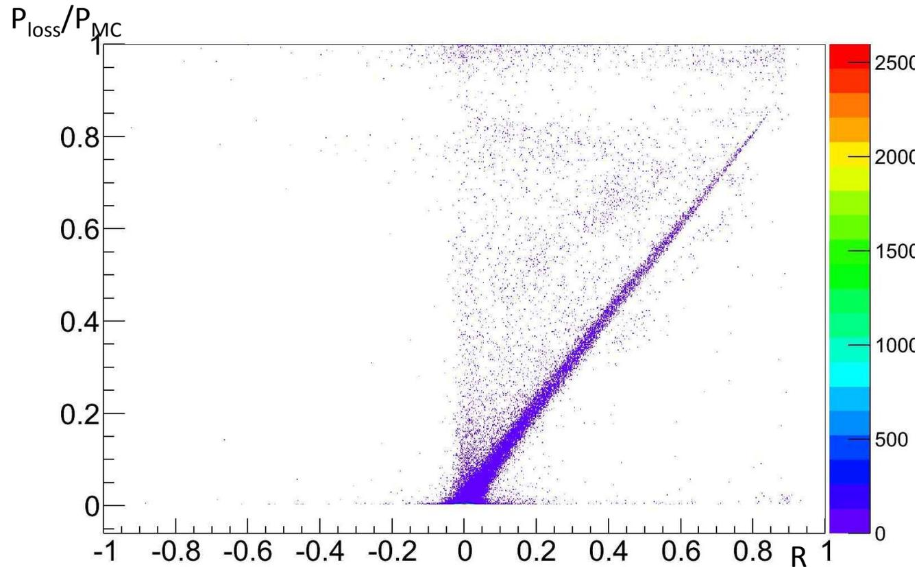
The KF reconstructs the momentum after  $\gamma$  emission with a good resolution.
