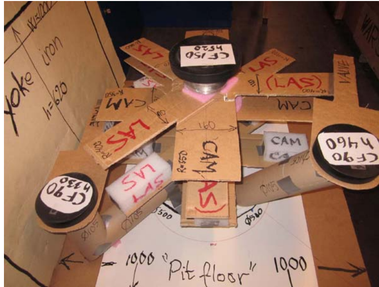
Fig.49. Side view from downstream. Pipes and “CF90” flanges for pumps (in two possible configurations). Heights of flanges above the floor are given.
