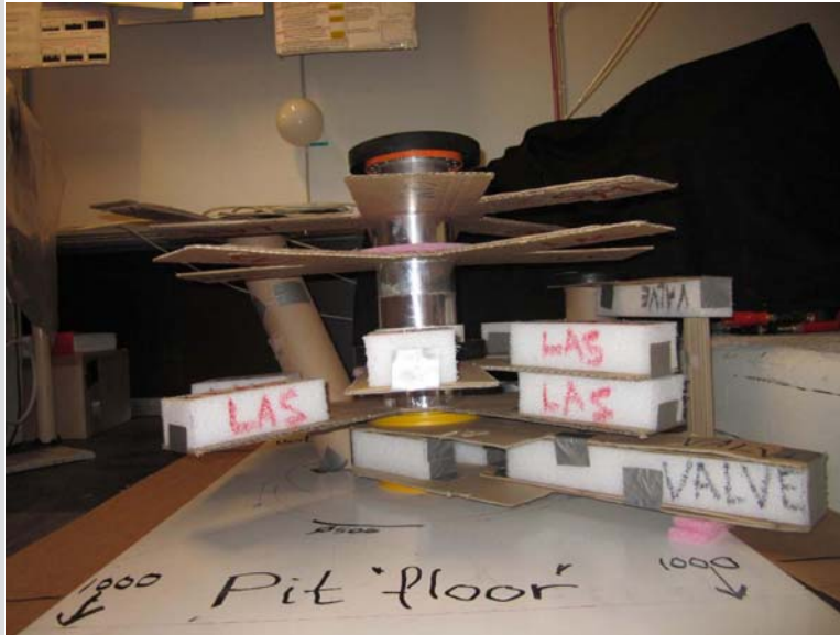
Fig.25. Floor view from upstream. Poor space to connect PTR section above DN160 valve. Yellow spacers have H=20\text{mm} .
