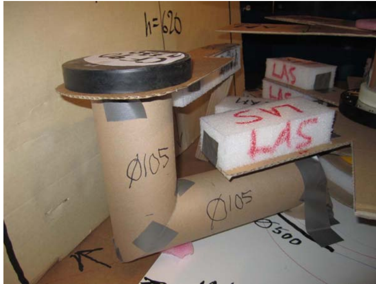
Fig.53. View from downstream. The S-shaped pipe for pump makes it possible to have a pump in this quadrant.
