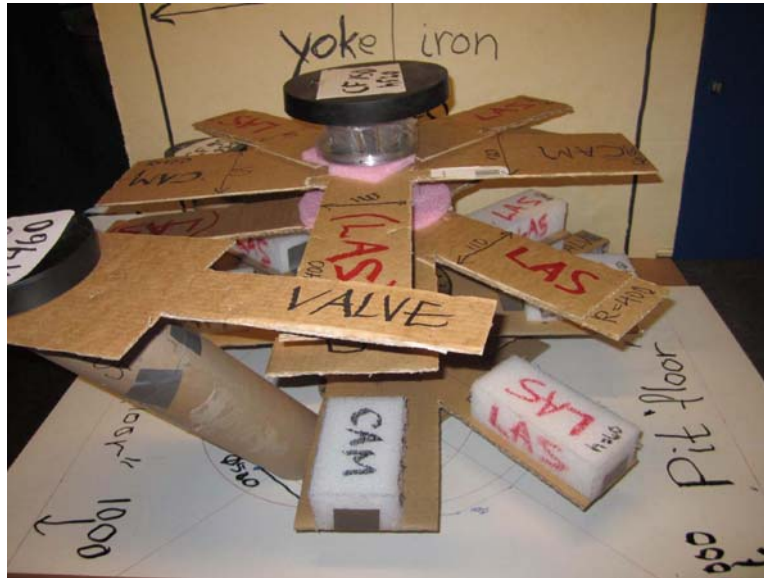
Fig.47. Side view from left. Valve “shaft” collide with camera/laser (at this height). To avoid this, the valve should move up further about 100 mm.
