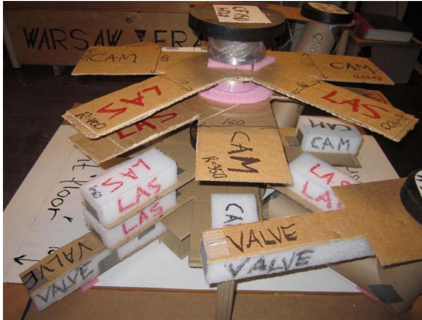
Fig.31. Side view from right. Detection levels and shafts of valves VAT S12 DN160 (down to the left) and DN100 are seen. The full height of a detection level is \approx 60\text{mm} .
