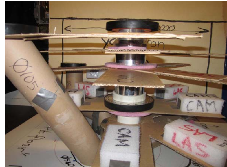
Fig.48. Side view from left. The bottom of the detection levels are shown by the corrugated cardboard sheets. On the lower two levels, foam plastic blocks illustrate the sizes of cams and lasers. The full height of a detection level is \approx 60 mm.
