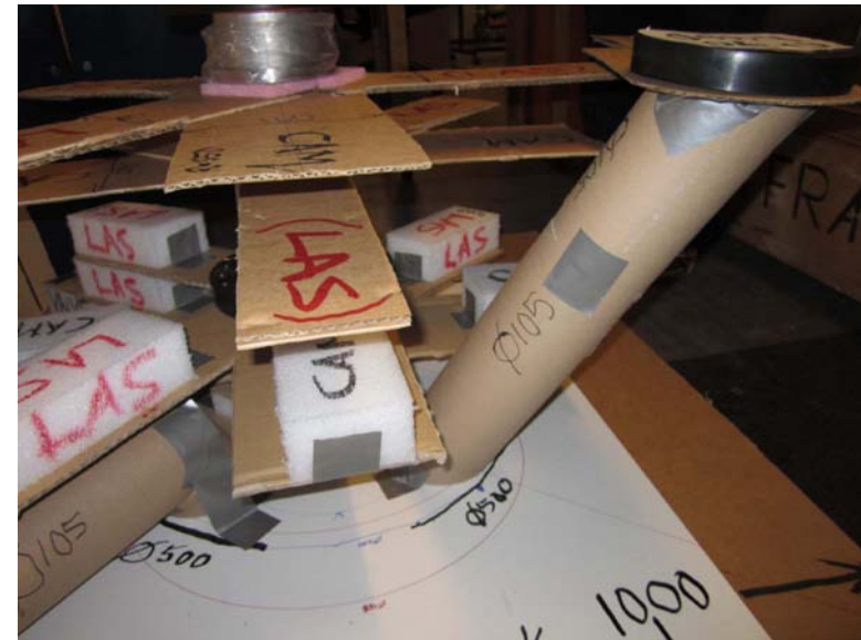
Fig.54. View from downstream. A pipe inclined 30 degrees is possible in this quadrant but a pump (and valve) must be placed very high, sticking up above the pit.
