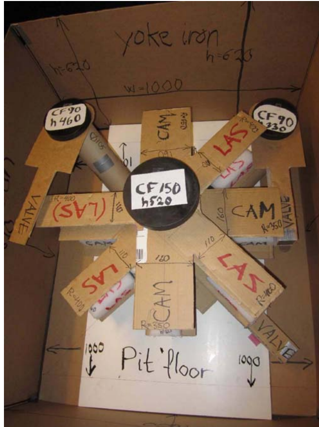
Fig.59. Top view from upstream. Pit W=1m L=1.2 m H=0.62m. Downstream left quadrant is “free” for tilted straight pump pipe.
