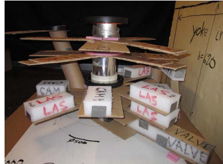
Fig.45. Side view from upstream. The bottom of the detection levels are shown by the corrugated cardboard sheets. On the lower two levels, foam plastic blocks illustrate the sizes of cams and lasers. The full height of a detection level is \approx 60\text{mm} .
