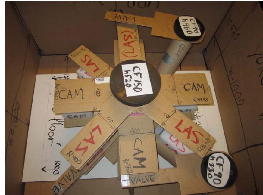
Fig.65. Top view from right. Pit W=1m L=1.2 m H=0.62m. One quadrant “free” for straight pump pipe. “CF150” flange for connection to pellet generator and “CF90” flanges for connection to pumps (in two possible configurations). Heights of flanges above the floor are given.
