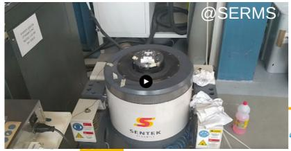
Before and after the two environmental tests high resolution pictures of the grid were taken and the ASICs were tested electronically → no differences were found
