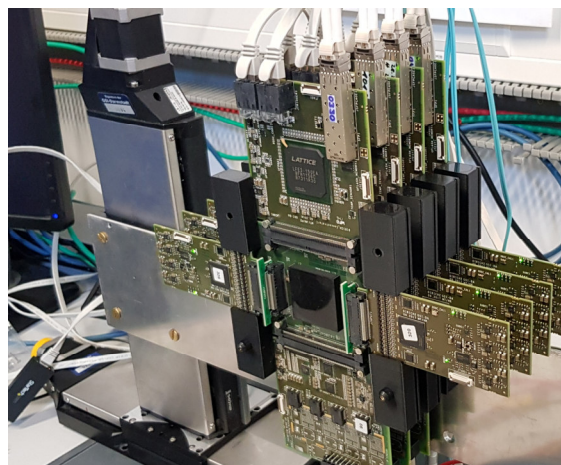
Figure 10: Four-layer beam telescope system with LGAD ultrafast silicon detectors installed at GSI (from DTS-ST3).
