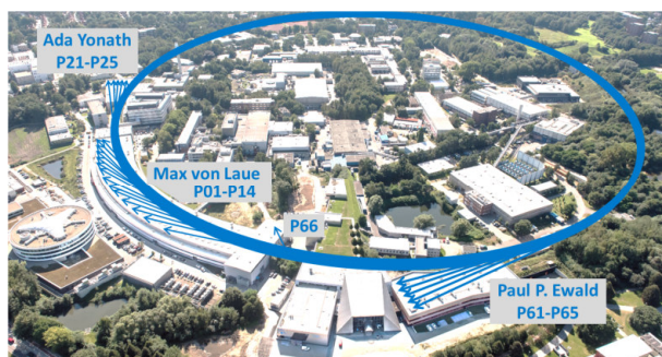
Figure 7: View of the PETRA III storage ring (blue ellipse) with the three experimental halls. Beamlines are sketched as blue arrows.
