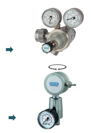
New **HP 105** Precision Pressure Regulator -compact construction by best control mode-A two-stage cylinder pressure regulator with maximum constancy of the set outlet pressure. The two-stage design with integrated inlet pressure compensation ensures a constant outlet pressure even with large changes at the inlet pressure.
