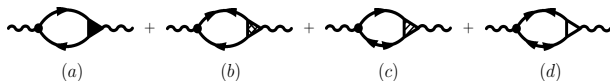
Figure: The sum of polarization tensors contributing to the vector-current neutrino emission rate. Note that the diagrams b , c , and d are specific to the superfluid systems and vanish in the unpaired state.
