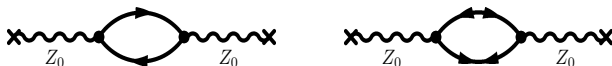
Figure: The two diagrams contributing to the polarization tensor of baryonic matter, which defines the axial vector emissivity. The “normal” baryon propagators for particles (holes) are shown by single-arrowed lines directed from left to right (right to left). The double arrowed lines correspond to the “anomalous” propagators F (two incoming arrows) and F^+ (two outgoing arrows).
