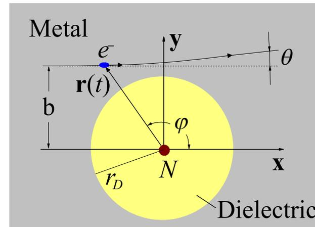
A new method of obtaining of aligned nuclei in *a crystal of ionic insulator*, which is cooled to cryogenic temperatures. Orientation is a result of inelastic scattering of the conduction electrons ( $e^-$ ) of the *metallic covering* of *sample* from the nuclei ( $N$ ). (E.Tkalya, *Submitted to PRC*)
