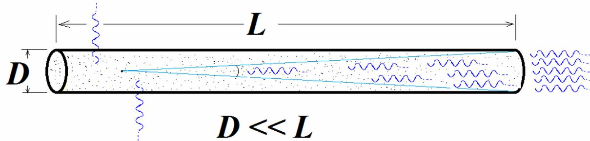
$\chi = 3 \text{ cm}^{-1}$ ,  $D = 0.1 \text{ mm}$ ,  $L = 5 \text{ cm}$ , the gain  $\exp(\chi L) \approx 10^6$
