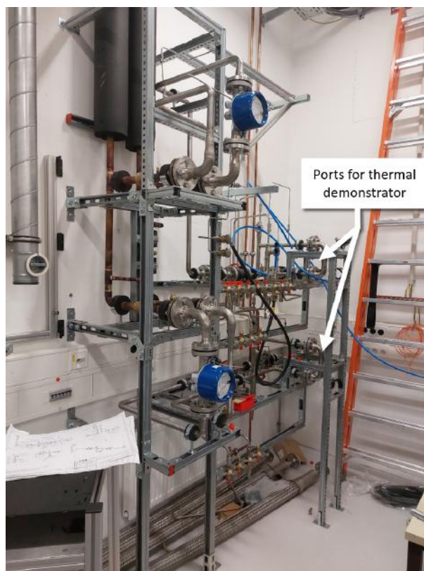
Figure 11: The cooling test rig
