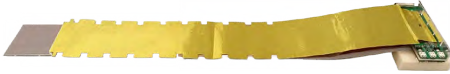
Figure 1: STS Module comprising a double-sided silicon micro-strip sensor (left), ultra-thin microcables (middle) and a pair of front-end electronics boards (right)
