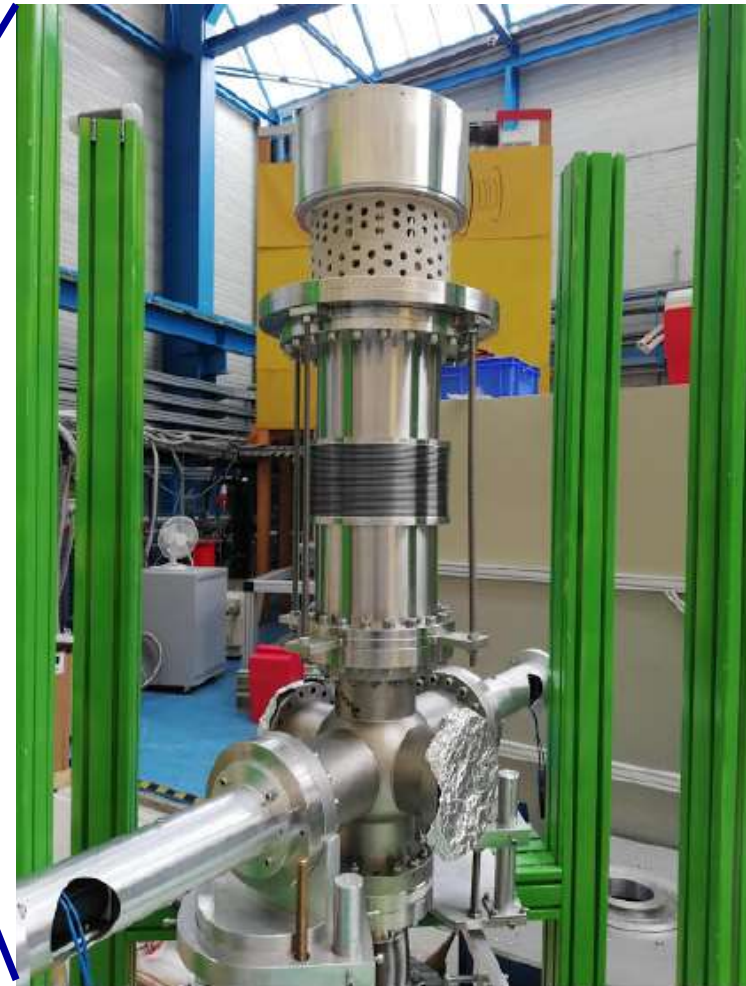
Test setup with cryovalve
