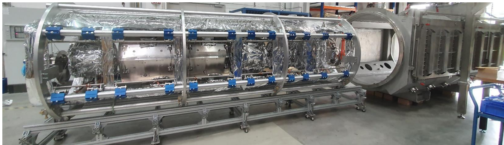
Acceleration string mounted inside transport frame
