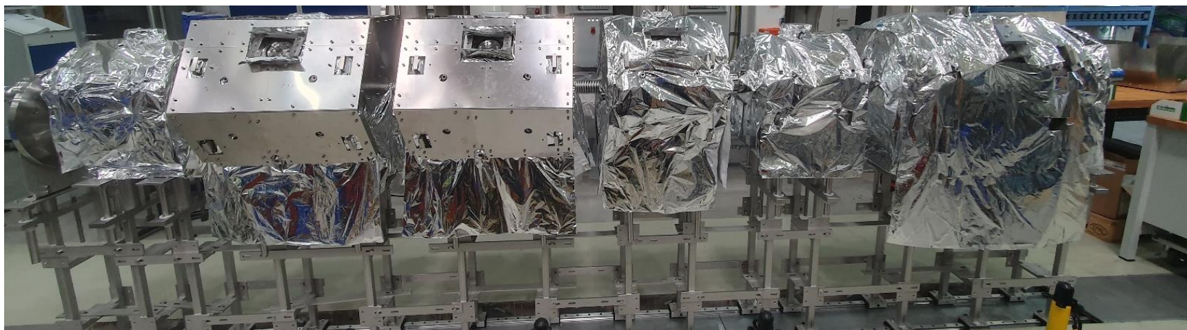
Acceleration string mounted on individual trolleys
