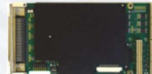
Reconfigurable FPGA-Modul with 64 or 32 Differential-I/Os
