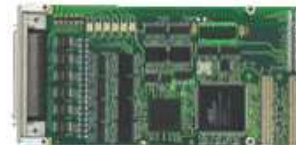
6-Channel SSI-Interface, Incremental encoder 24V Inputs
