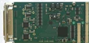
16/8-times 16-bit ADC, 8/4-times 16-bit DAC and 14-times TTL Digital I/O
