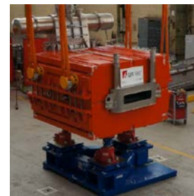
ELYTT (Spain) SFRS sc dipole magnets
